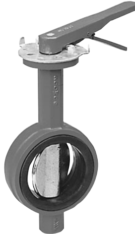
FIGURE 8.13 A wafer-type butterfly valve with cast iron body, stainless steel shaft, 10-position lever, and elastomeric seats. The valve is sandwiched between two flanges. Note that the elastomeric seat serves as a flange gasket. No additional gasket is required. Photo provided by Watts Regulator Company.
