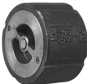
FIGURE 8.9 A cast iron silent check valve used to prevent water hammer due to pump shut down. Photo provided by Watts regulator Company.
