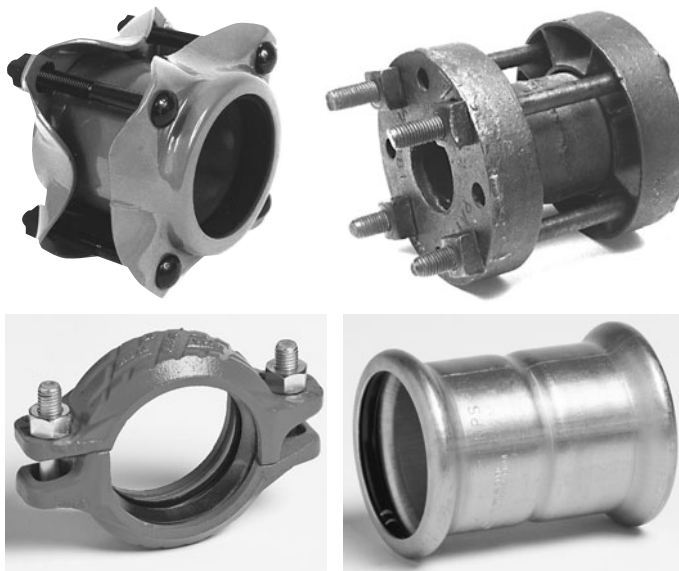
FIGURE 6.5 Mechanical joints, left-to-right, top-to-bottom: Dresser Style 38 coupling, Dresser mechanical coupling manufactured in 1890, Victaulic Style 77, Victaulic Style 597, which crimps to the adjoining pipe with a special rolling tool. Credits: Style 38 and 1890 Couplings, Dresser Piping Specialties, Dresser Inc., Victaulic images reprinted with permission of Victaulic Company.
