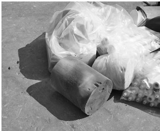
FIGURE 16.3 A cylindrical foam pig that has been used to wipe a chemical line.
