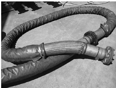
FIGURE 8.41 A corrugated stainless steel hose. Note the exterior braiding which acts as an axial restraint.
