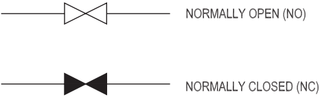
FIGURE 10.6 Normally closed valves are represented with the valve outline shaded.
