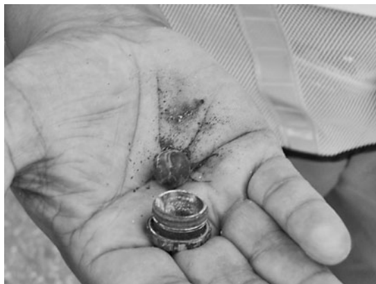
FIGURE 15.2 Check valve internals corroded due to exposure to sea water flooding. These valves were on gas utility drops in an industrial facility.
