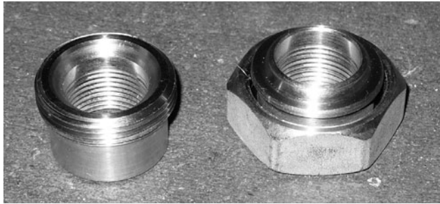
FIGURE 7.19 A disassembled threaded union showing ground seat and metal-to-metal seal.
