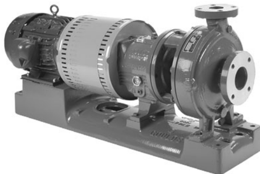
FIGURE 11.6 A typical end suction centrifugal pump with motor and coupling mounted on a cast iron baseplate. Note the grout hole to assist in placing grout under the baseplate. Cast iron is often used for baseplates due to its excellent vibration dampening properties. ITT Goulds Pumps. All rights reserved.
