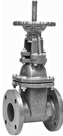
FIGURE 8.1 Outside Stem & Yoke flanged gate valve with rising stem and epoxy coated cast iron body. Photo provided by Watts Regulator Company.
