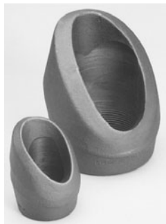
FIGURE 7.25 A Latrolet® branch connection fitting for turning a straight run into a lateral. 1 The attached fitting may be butt-welded, socket welded, or threaded.
