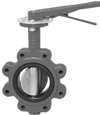
FIGURE 8.14 A lug-type butterfly valve with cast iron body, stainless steel shaft, 10-position lever, and elastomeric seats. The seat acts as a flange gasket. Photo provided by Watts Regulator Company.
